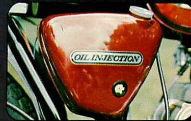
Bridgestone's proven full-time oil injection plus pressure lubrication of engine bearings means added engine life and performance.
