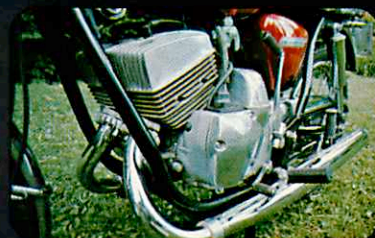
The engine—40 horsepower. Aluminum alloy cylinders, chromed bores; 4 main bearings; oil injection; six speed transmission.
